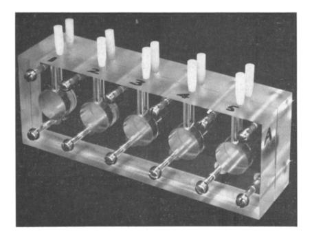
The device shown in the Figure was fabricated from 2 pieces of  $8\times3\times1$  inch plastic. Five 1 inch diameter wells were 'end-milled' into each piece to a depth of 1/2 inch. The dialysis membrane was placed between the 2 pieces, and the device was assembled with 12 bolts and wing nuts.
